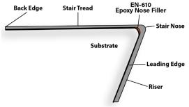
Overlap the stair tread above the riser with the riser while ensuring that riser toe is not over-compressed. Using the leading edge of the stair tread as a guide, a divider or a marking tool is needed to scribe the riser. Use a suitable knife to trim riser along the scribe mark.
